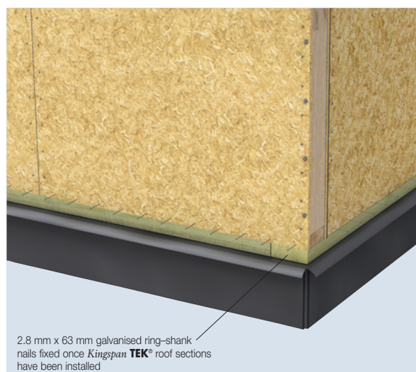
Figure 34 Fixing Ground Floor Wall Panels to Bottomplate
