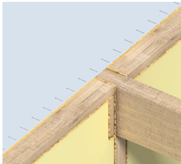
Figure 21b Cross Section Through Wall Showing Installed Beam
